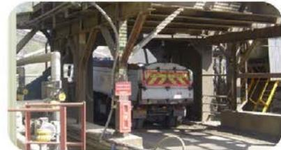
**Hot Mix Asphalt (HMA)** – Generally produced at a temperature between 150°C and 180°C.
