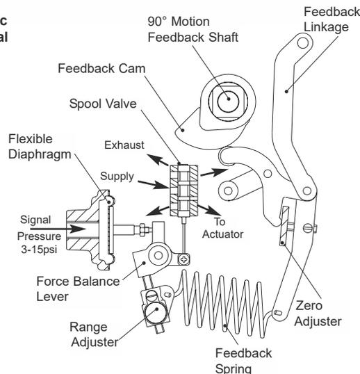
The AP positioner moves an actuator to a position set by a 3-15psi control signal and holds it there. Its features are:
